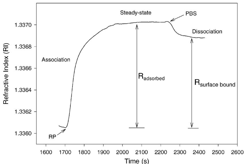
Fig. 2. Change in refractive index with time for the assembly of a single electrostatic layer of RP (10 mg/ml in PBS, flow rate  $80\ \mu\text{l}/\text{min}$ ).
