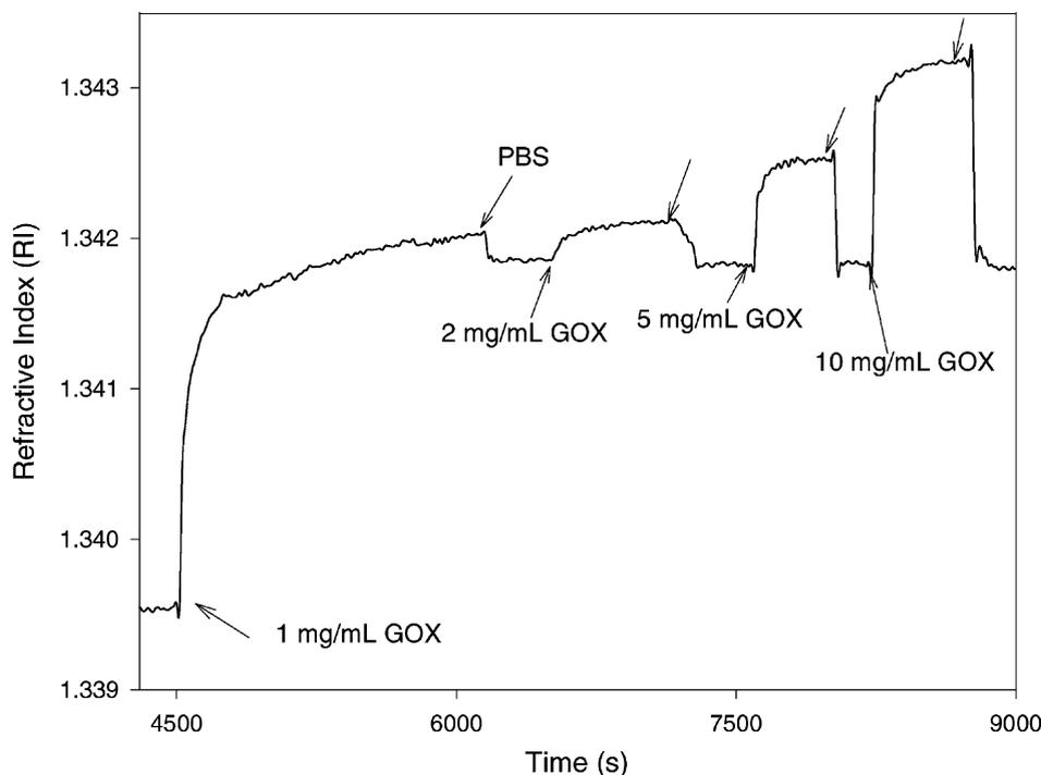
Fig. 4. Determination of the minimum GOX concentration needed for complete surface saturation. Flow rate  $80 \mu\text{l}/\text{min}$  was employed. Each equilibrium state was followed by flushing with PBS. These steps are denoted by arrows.
