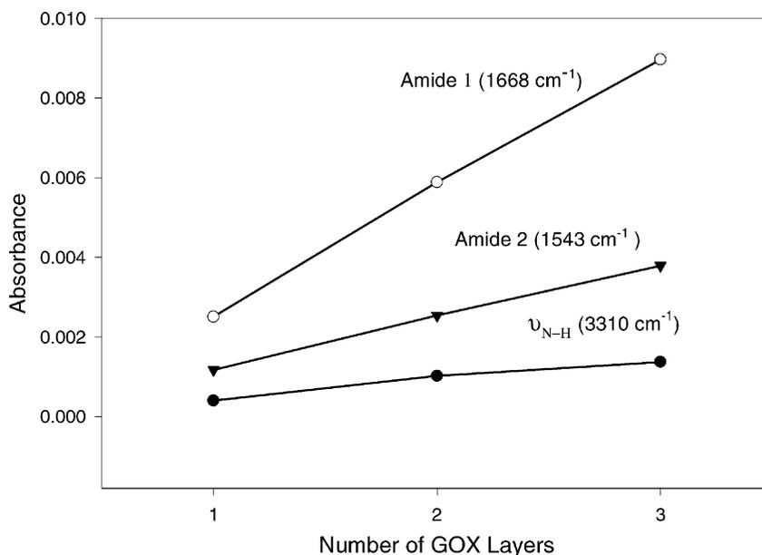
Fig. 7. Plot representing absorbance in the amine stretching and amides 1 and 2 regions as a function of number of layers.
