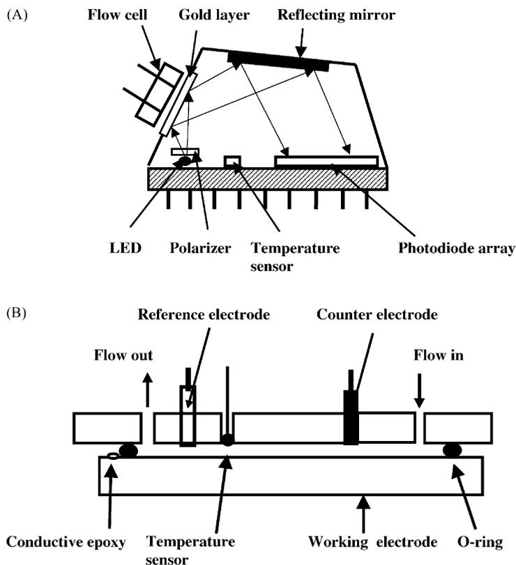
Fig. 1. (A) Schematic of the miniature Spreeta sensor. (B) Cross-sectional view of the test cell used for combined SPR/electrochemistry experiments.
