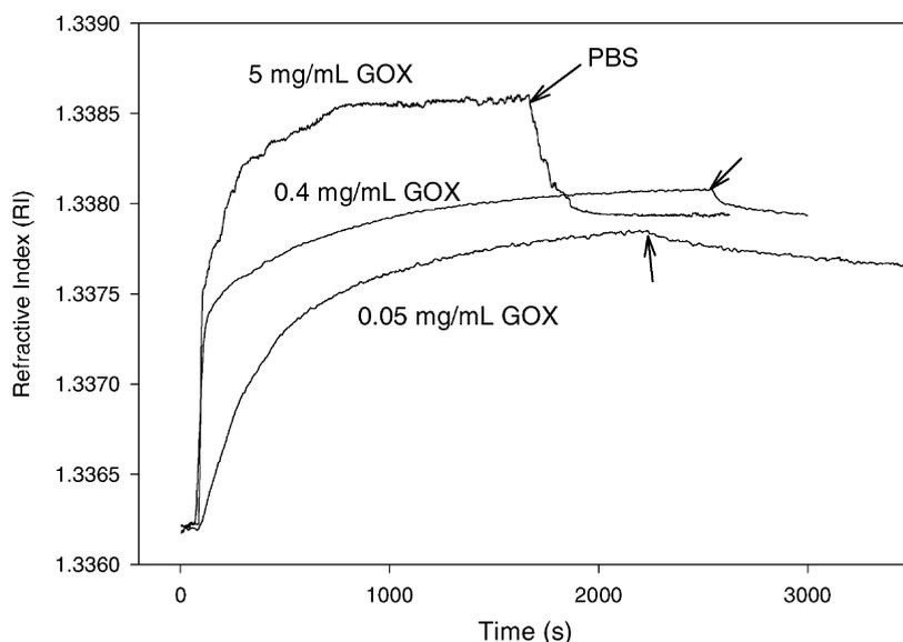
Fig. 5. Affinity constant determination for the binding of GOX (flow rate  $80 \mu\text{l}/\text{min}$ ) with surface-bound RP layer. Arrows denote injections of PBS wash solution.
