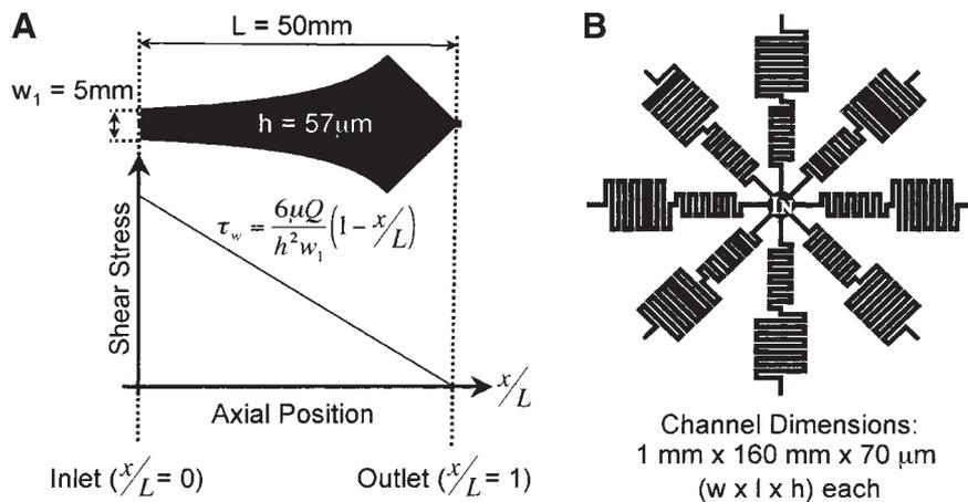
**Figure 1.** Schematics of the two microfluidic chambers used in this study: (A) Hele-Shaw flow chamber and its shear stress profile, as well as the (B) parallel flow chamber.
