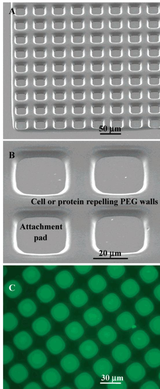
**Figure 2.** Micrographs of PEG microwells on glass. (A) SEM image of the high-density array of  $30 \times 30$   $\mu\text{m}$  hydrogel microwells with  $20$ - $\mu\text{m}$  cell-resistant PEG side walls ( $\times 270$ ). (B) Higher-magnification ( $\times 900$ ) SEM micrograph of the hydrogel microstructures. (C) Fluorescein-labeled collagen coating the bottom of  $30 \times 30$   $\mu\text{m}$  wells ( $\times 400$ ).
