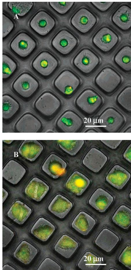
**Figure 5.** Viability of the cells confined within PEG microwells with  $30 \times 30 \mu\text{m}$  individual dimensions as determined by the Live/Dead assay. Both micrographs were obtained at  $\times 400$  using confocal microscopy. (A) 3T3 fibroblasts after 12 h of incubation. (B) Primary hepatocytes after 24 h of incubation.
