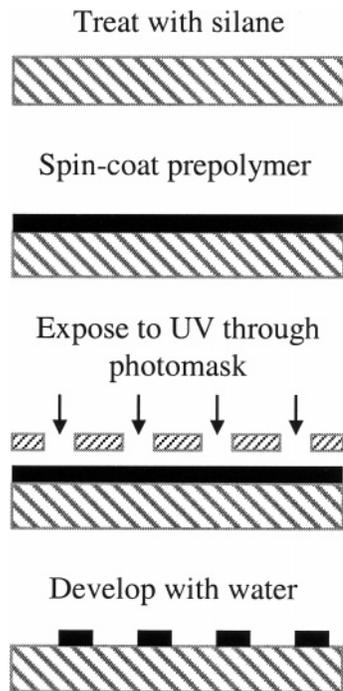
**Figure 1.** Process flow for the fabrication of PEG hydrogel microstructures.
