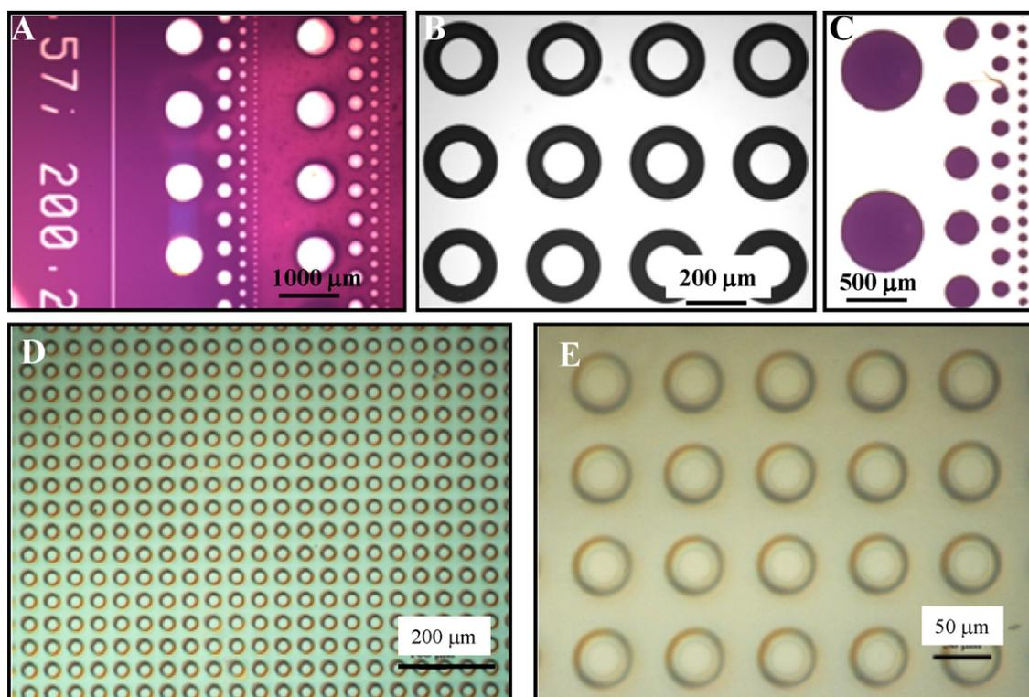
**Fig. 3.** Micropatterning of hydrogels on thiol-silane-modified glass surfaces. (A–C) Heparin/PEG hydrogels stained with toluidine blue and (D–E) PEG hydrogels microstructures.
