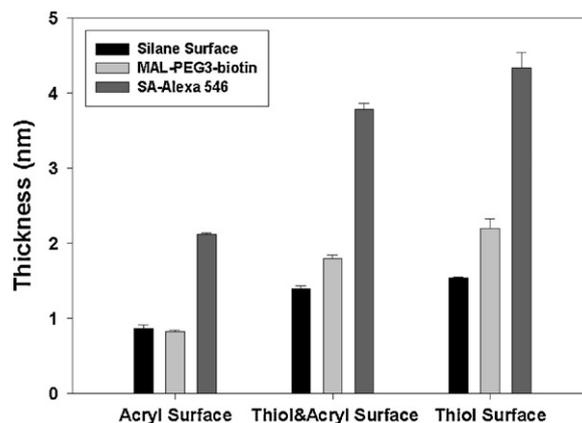
**Fig. 2.** Characterization of surface modification using ellipsometry. Adsorption of linker (Mal-PEG-NHS) caused a thickness change of ~0.5 nm on mixed-silane and thiol-silane surfaces, but no difference on acryl-terminated silane. In addition, significantly more streptavidin adsorption was observed on thiol-terminated silane (2.14 nm layer) vs. acryl-silane (1.25 nm layer).
