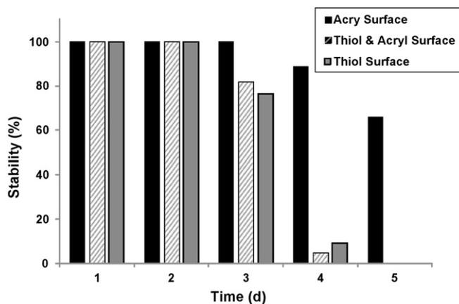
**Fig. 4.** Stability of hydrogel micropatterns on thiol-, mixed-, and acryl-silane functionalized surfaces in aqueous solution. The stability was quantified by calculating the ratio of the number of remaining hydrogel microwells to the total number of hydrogel microwells.
