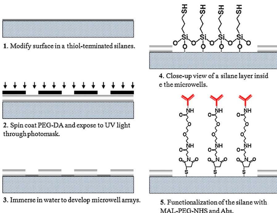
**Fig. 1.** Process flow diagram for hydrogel micropatterning and protein attachment. PEG-hydrogels were directly fabricated on thiol-silane surfaces using photolithographic methods. Thiol groups remain on the surface of the unpolymerized regions, allowing for covalent linking of proteins.
