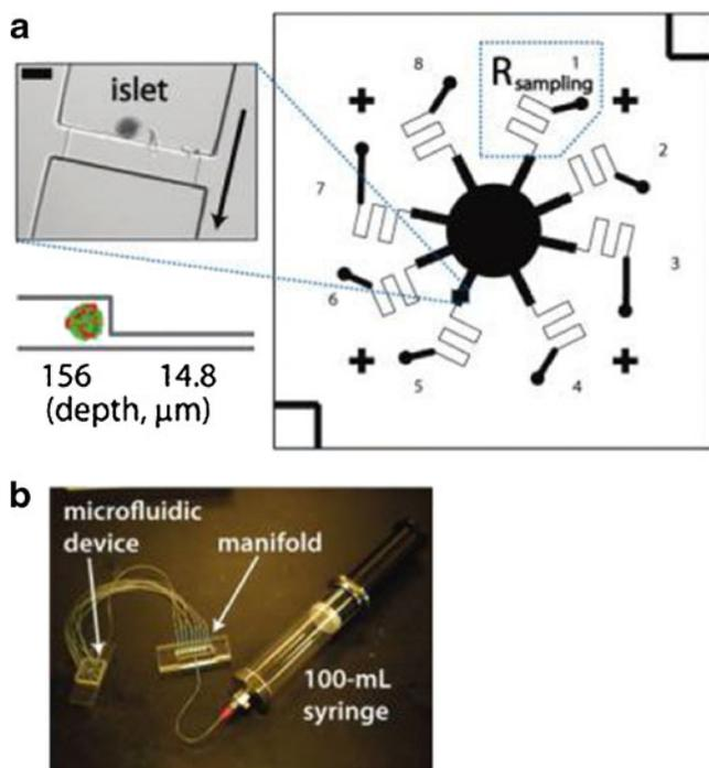
**Fig. 5** Passively operated microfluidic device for islet secretion sampling and imaging. **a** Device layout, including an image of a trapped islet. **b** Hand-held apparatus for secretion sampling with no electrical components. The figure is based on information presented in [94]
