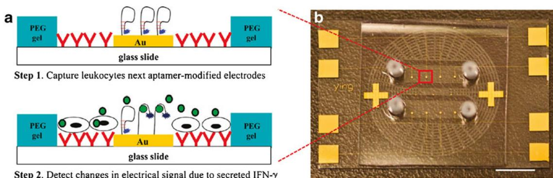
**Fig. 2** **a** Schematic of the sensing area layout. Au electrode arrays fabricated on glass slides are surrounded by PEG hydrogel and incubated with T cell-specific antibodies. Upon injection of blood, leukocytes are bound on Ab-modified glass regions next to aptasensors. Cytokine release is detected at the aptamer-modified electrodes by an
