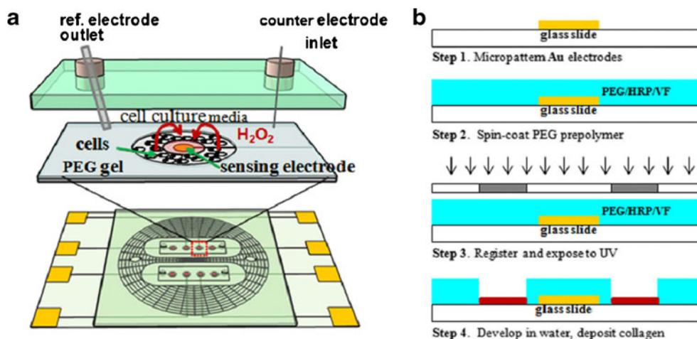
**Fig. 4** **a** Upper panel: schematic of a single electrode for detection of cell-secreted  $\text{H}_2\text{O}_2$ . Macrophages are captured on a micropatterned surface in the vicinity of sensing electrode. The sensor consists of an HRP-carrying hydrogel disc immobilized on top of a 300- $\mu\text{m}$ -diameter Au electrode. Each channel constituted an electrochemical cell with Ag/AgCl flowthrough reference and platinum wire counter electrodes
