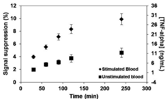
**Fig. 4** Monitoring of TNF- $\alpha$  release from whole blood using aptamer modified electrodes. PMA/ionomycin was used as the stimulant. The calibration curve was used to convert signal suppression into TNF- $\alpha$  concentration (right y-axis).
