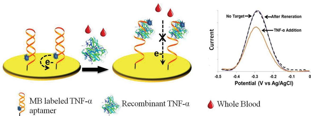
**Fig. 1** (A) Schematic representation of the TNF- $\alpha$  aptasensor with Methylene Blue (MB) as a redox label. In the absence of target, aptamer hairpins remain folded with MB reporters in proximity to the electrode, ensuring efficient electron transfer ( $e^-$ ) and a measurable faradaic current. Upon target binding, the redox tag moves further away from the electrode and the redox current decreases. (B) This RNA aptasensor can be fully regenerated using 7 M urea buffer.
