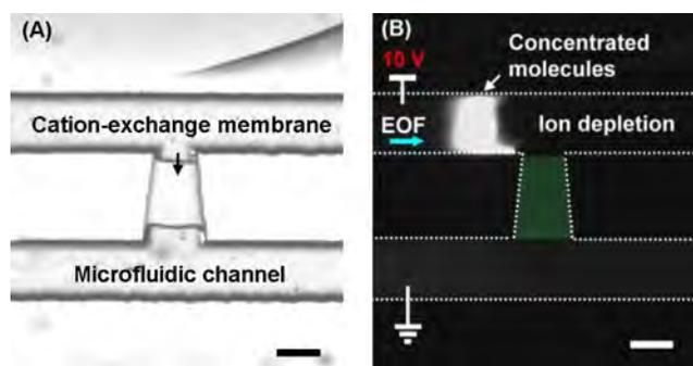
FIG. 8. (a) Optical microscopic image of a charge-selective membrane based preconcentrator. (b) Concentration of fluorescently labeled molecules taking place 10 s after applying a voltage bias of 10 V. The scale bars represent 50  $\mu m$ .
