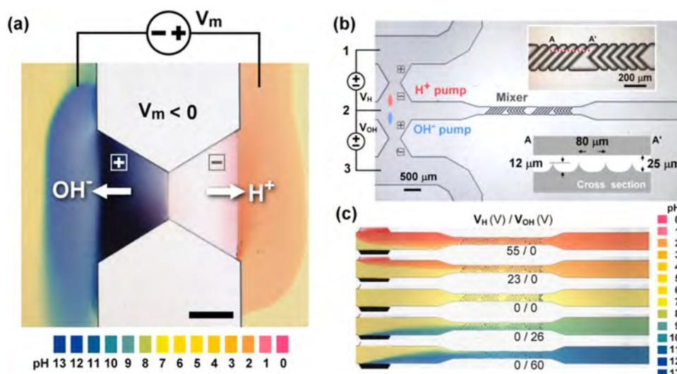
FIG. 7. An on-chip bipolar membrane  $pH$  actuator. The image in (a) shows how a DC field across a bipolar membrane can dissociate water and generate protons and hydroxyl ions at a controllable rate. Two such bipolar membranes are fabricated up stream of a flow channel and the protons/hydroxyl ions are mixed by a static mixer into a buffer of a specific  $pH$  between 2 and 10 in (b). The mixed streams are shown in (c) with a color chart for the universal  $pH$  dye.
