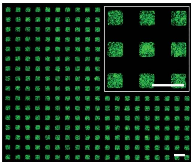
**Fig. 4** 20 µm nanobead dot array with inset showing an enlarged view. Bars are 40 µm.
