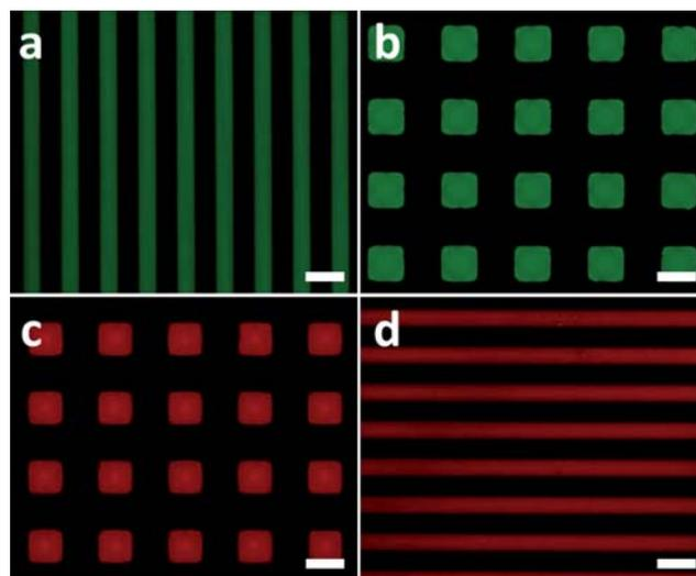
Fig. 3 Protein line array (a, d) of 10  $\mu\text{m}$  in width and dot array (b, c) of 20  $\mu\text{m}$  in side length. Bars are 20  $\mu\text{m}$ . Green patterns are BSA-FITC and red patterns are BSA-TR.
