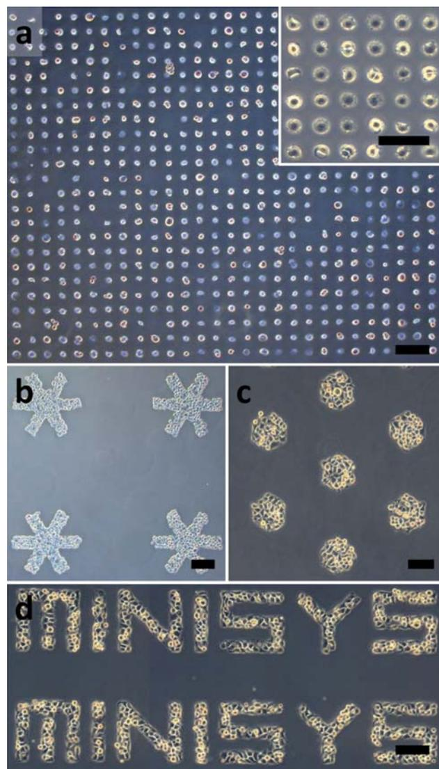
**Fig. 5** Single cell (a) and arbitrary cell patterns (b–d). Bars are 120 µm.
