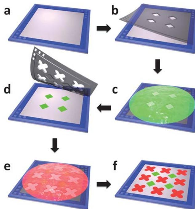
**Fig. 2** The fabrication of two-protein micropatterns using stereomask lithography. (a) Aligning frame with micropillars is laminated onto target substrate. (b) First stereomask is aligned with aligning frame using peg-in-hole method and laminated onto substrate. (c) BSA-FITC is incubated. (d) Second stereomask is aligned using the same method and laminated onto substrate. (e) BSA-TR is incubated. (f) Second stereomask is peeled off and two-protein patterning is complete.
