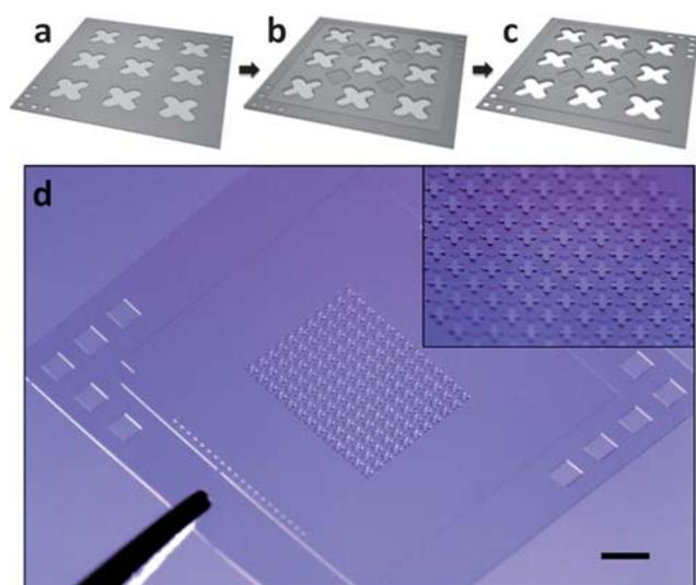
**Fig. 1** Schematic illustration of stereomask fabrication: (a) the first layer of dry film is photopatterned with cross-shaped through-windows; (b) the second layer of dry film incorporates both the through-windows and the diamond-shaped protective chambers; and subsequently (c) the dry film stereomask is developed in PGMEA and a macroscopic picture of stereomask with an inset showing a microscopic view of through-patterns and protective chambers (d). Bar is 1 mm.
