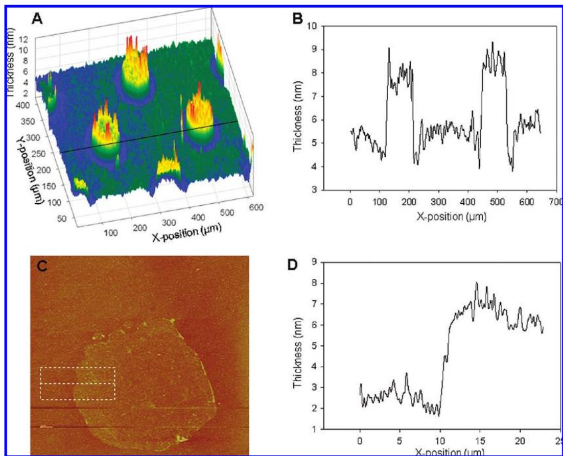
**FIGURE 4.** Imaging protein islands created by filling the recesses. (A) A topograph showing protein micropatterns on ITO using imaging ellipsometry with (B) corresponding cursor profile. (C) AFM micrograph and (D) corresponding surface profile of collagen pillars on ITO surrounded by PEG silane. The height of the collagen pillars from PEG silane calculated using imaging ellipsometer and AFM is  $\sim 3.5$  nm.
